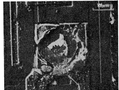
Fig.7 Enlarged micrograph of corroded Aluminum bonding pad
